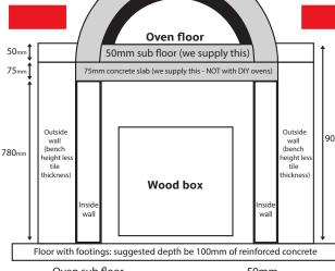
Oven sub floor 50mm Slab 75mm Sub floor and slab 125mm Bench height 905mm +/-Supporting wall for oven 780mm +/-Oven floor height on supporting wall 905mm +/-
