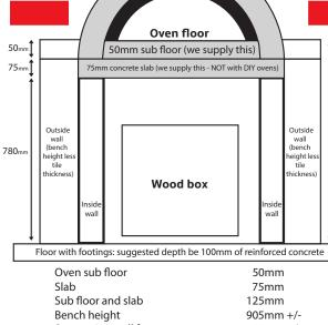
Supporting wall for oven 780mm +/-Oven floor height on supporting wall 905mm +/-
